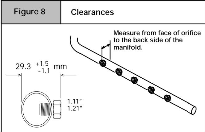
8. Reassemble all parts in reverse order as removed. Be sure to engage the main burner orifices in the proper opening in the burners.
