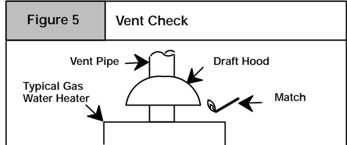
8. If improper venting is observed, the cause **MUST** be corrected.
