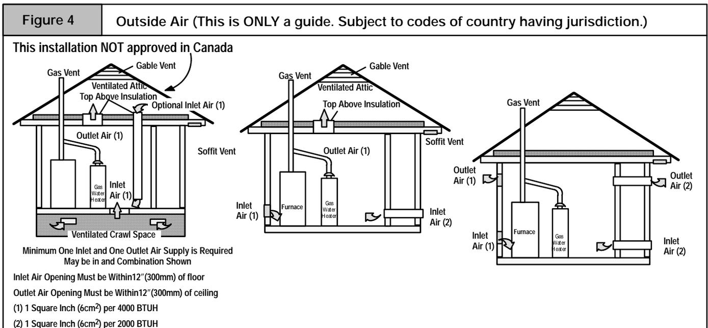
3. One opening **MUST** be within 12" of the floor and the second opening within 12" of the ceiling.
