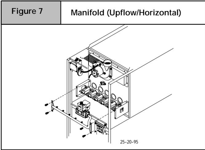
5. Carefully remove the manifold assembly.
