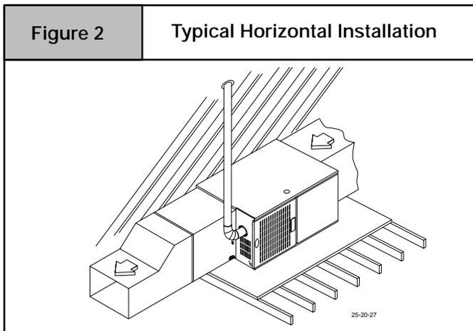
The following minimum clearances to combustibles **MUST** be maintained between the furnace and adjacent construction, as shown in **Figure 1**. **ONLY** the corner of the cabinet is allowed to contact the rafters (see **Figure 2**). All other clearances **MUST** be observed as shown in **Figure 1**.
