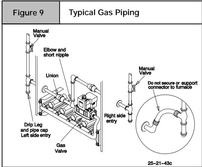
7. Use two pipe wrenches when making connections to prevent gas valve from turning.
