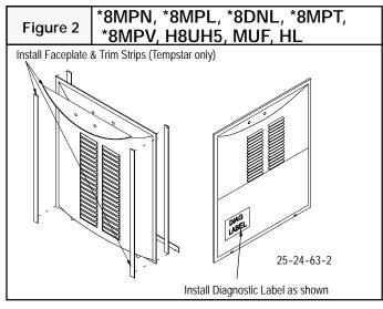
1. Place one Diagnostic Label on the bottom left corner of the sound shield installed on the backside of the door.
