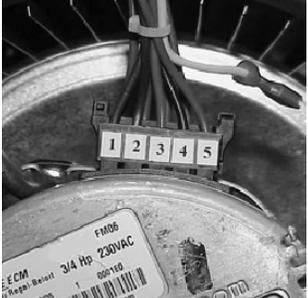
Verify that the proper blower speeds for heating and cooling are selected on the blower motor by removing the blower access panel and inspecting the blower motor. The motor has 4 speeds numbered "1", "2", "3", and "4". The wires for the speed selection are as follows:
