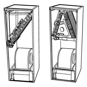
SLOPE COIL A-COIL
