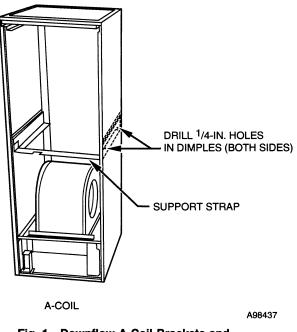
Fig. 1—Downflow A-Coil Brackets and Support Strap Location
