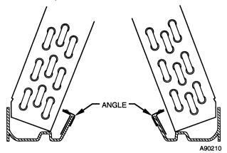
Fig. 2—Position of Angles on A-Coil
